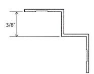
Modern Inside Corner creates a square and true termination point for cement panel siding at an inside corner.
