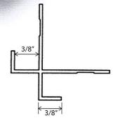
Modern Outside Corners create a straight, true and abuse resistant corner with exposed flanges that cover the vertical edges of the cement siding.
